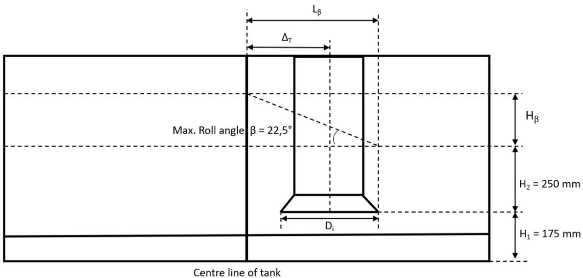
Figure 47: Dimensions relevant to calculate oil level reduction due to roll,  $H_\beta$ . Illustration: NSIA
