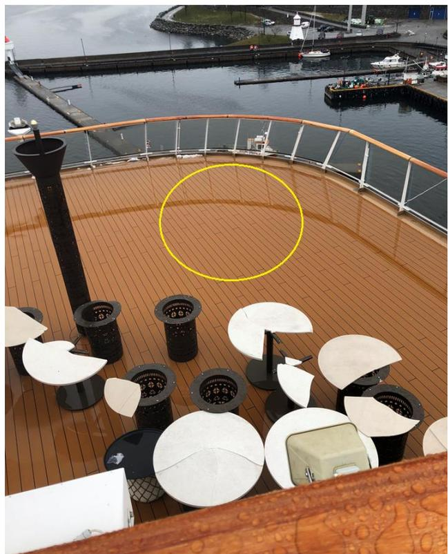
Figure 19: Secondary hoisting area, aft, deck 7. For safety reasons, this area was never used.
