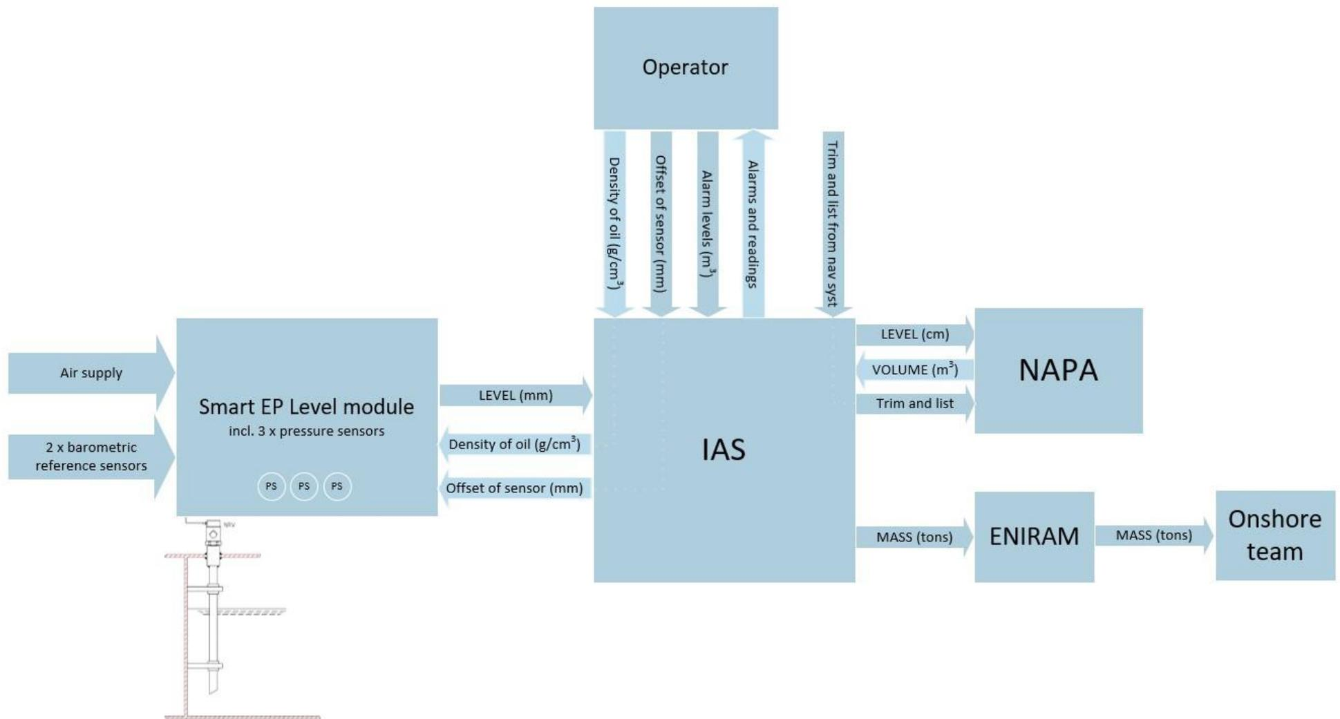
Figure 56: Functional block diagram, lube oil level remote monitoring system. Illustration: NSIA
