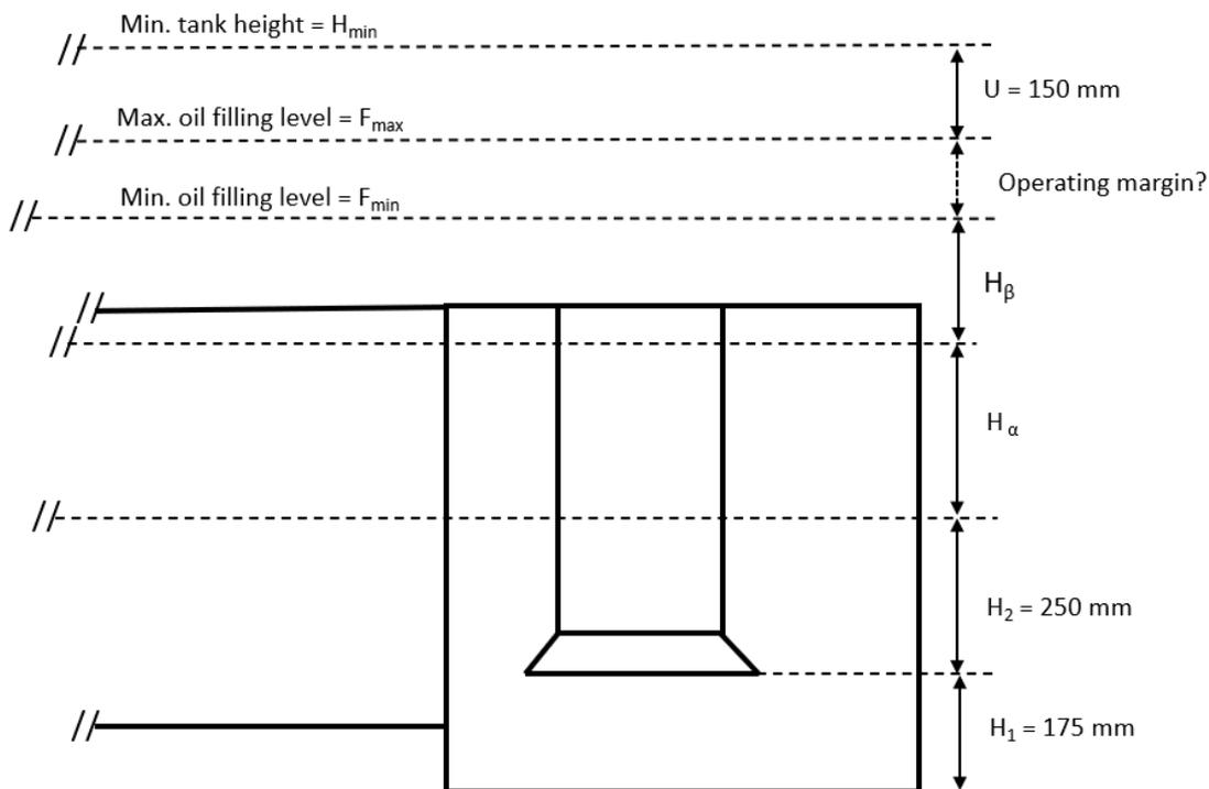
Figure 48: Minimum oil filling and tank height. Illustration: NSIA
