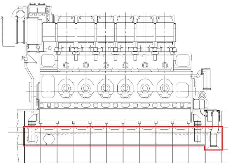
Figure 31: Diesel engine and sump tank (indicated in red) side view. Source: MAN/NSIA
