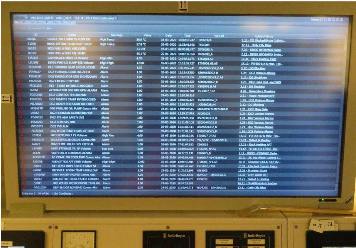
Figure 58: Alarm list as presented to the operators in the ECR. Photo: NSIA
