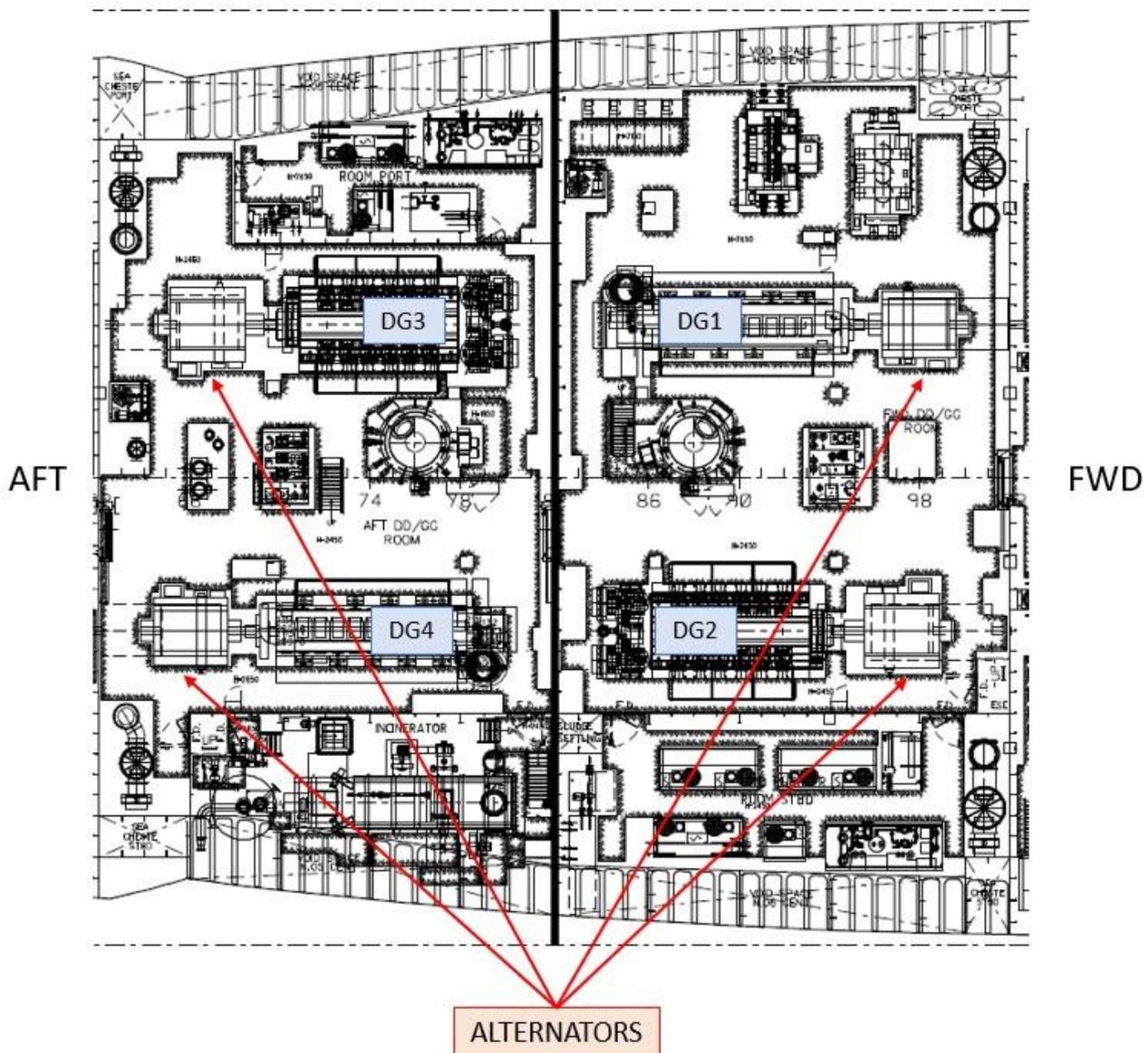
Figure 28: Extract from the vessel's General Arrangement, showing the positioning of the DGs. Illustration: Fincantieri/NSIA
