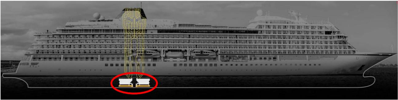
Figure 29: Viking Sky in profile, showing location of the DGs and the lube oil sump tanks. Illustration: Adobe Stock/Fincantieri/NSIA
