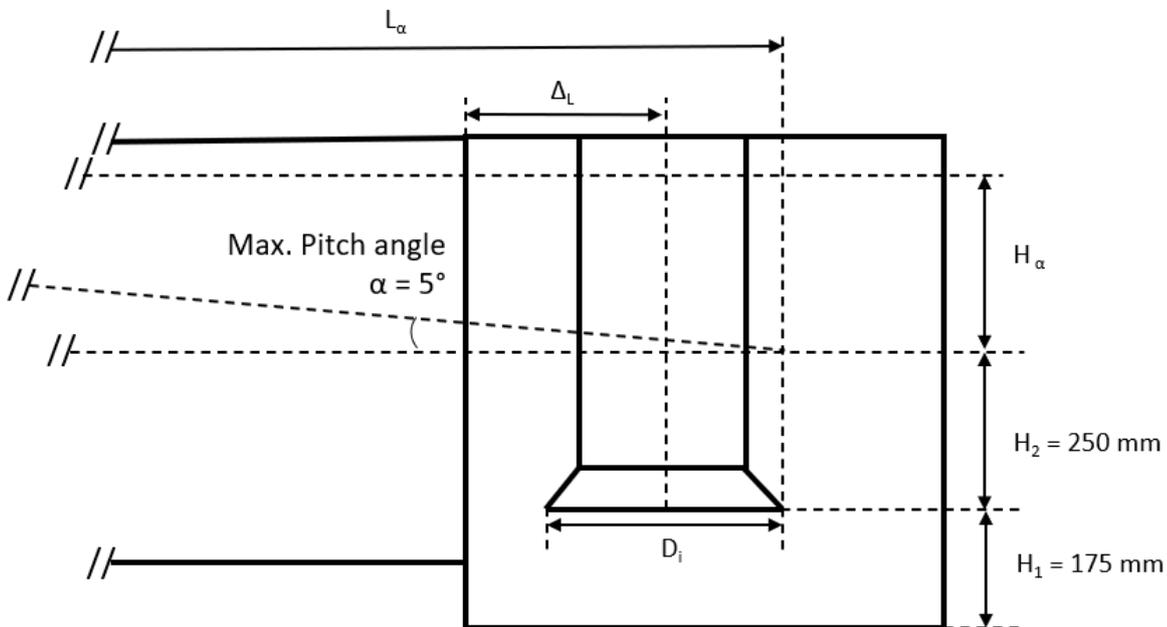
Figure 46: Dimensions relevant to calculate oil level reduction due to pitch,  $H_\alpha$ . Illustration: NSIA
