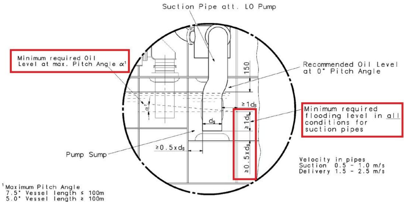
Figure 38: MAN project guide lubricating oil suction pipe detail. Extract: MAN
