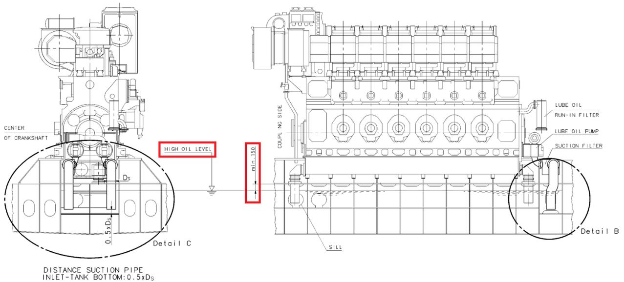
Figure 37: Extract from the MAN project guide showing the high oil level to be min 150 mm below the tank top. Extract: MAN
